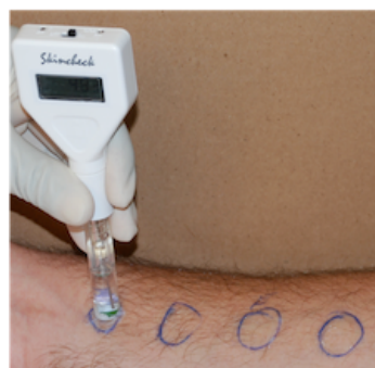
Fig. 3: Skin pH was measured using Hanna, HI99181 Skin pH meter following application and rinse-off of the washes on the forearms.
