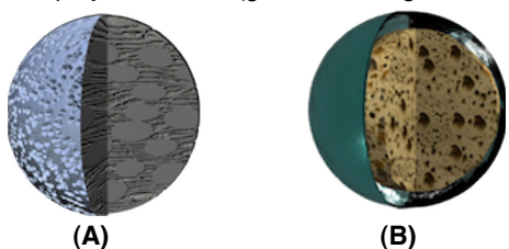
Fig. 1: Structure of HydroSal™ core with a temporarily evaporated shell (A), and with the outer shell intact (B).
